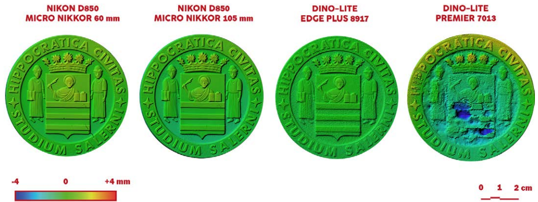
Fig. 6. Digital Elevation Model, obtained in the Agisoft Metashape software environment, of the models returned by the systems under comparison. Elaboration by the author.
