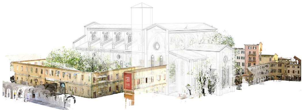
Church of Sant'Agostino - Padua: overlapping of the BIM model of the historical reconstruction with the current digital survey of the area. Elaboration by the author.
