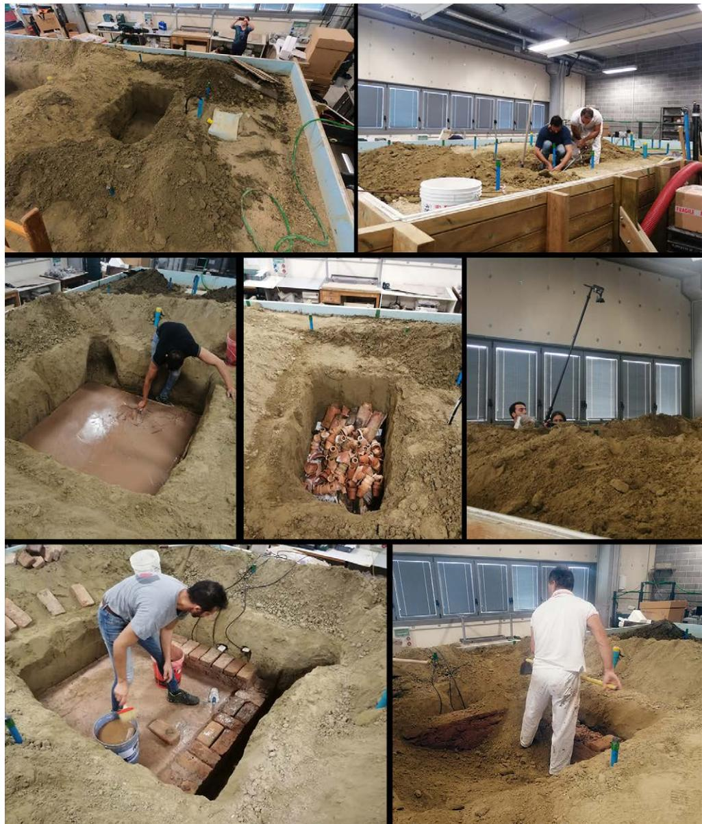
Fig. 2. Sequence of excavation operations, construction of the artefact's, and subsequent coverage with sandy material.
