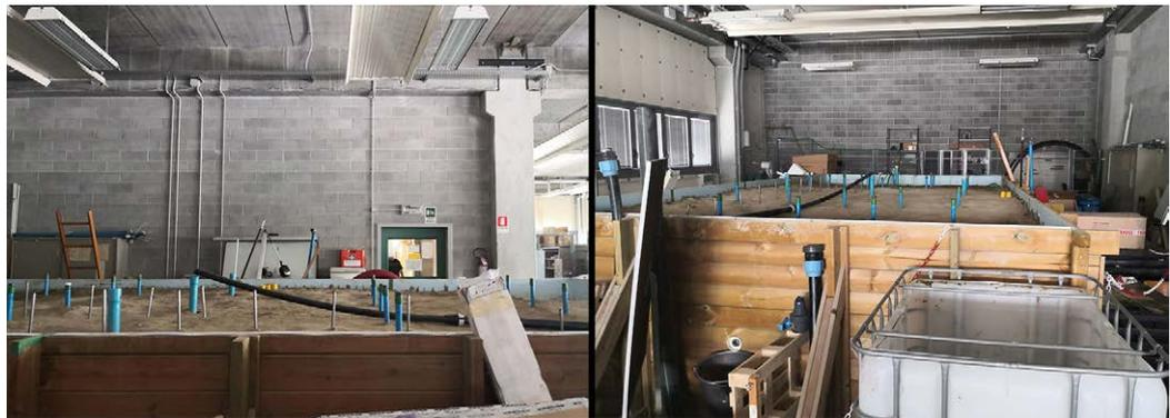
Fig. 1. Basin of 50 m<sup>3</sup> containing sediments from the Ferrara plain before the start of operations.
