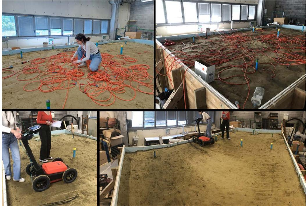
Fig. 3. Acquisitions with electrical resistivity tomography (top) and Ground Penetrating Radar (bottom).
