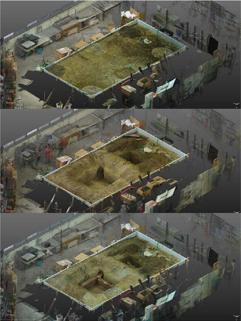
Fig. 7. View of the point cloud in the three successive phases of the survey (Trimble RealWorks).
