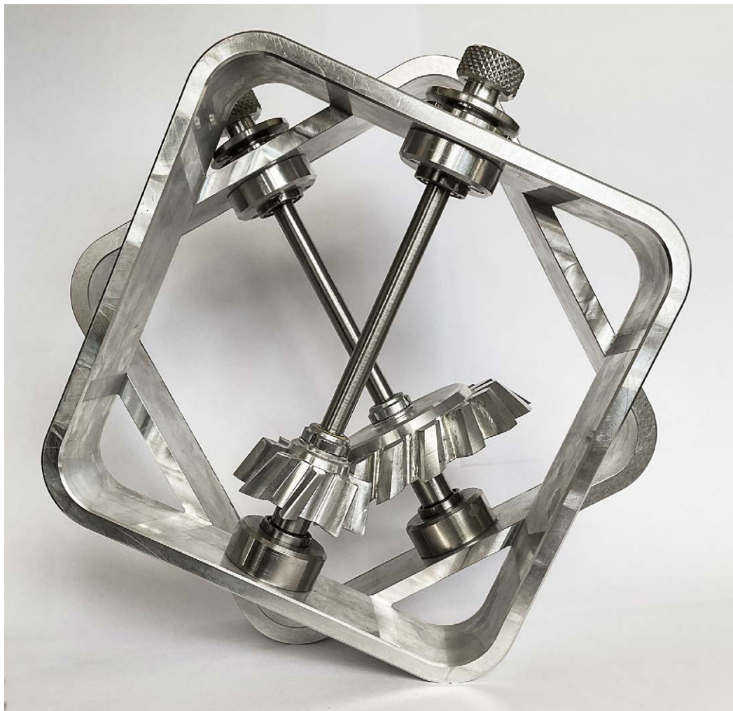
Prototype made of aluminum and steel. The use of portions of hyperboloids far from the point of minimum distance between the axes of revolution induces axial loads that are dissipated through the use of angular contact ball bearings, mounted in an opposing configuration.
