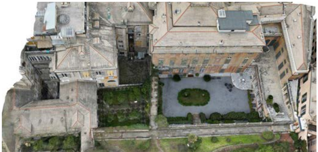
Fig. 11. Aerial photogrammetric survey of the palace and garden - 3d model with texture. Elaboration by the authors.
