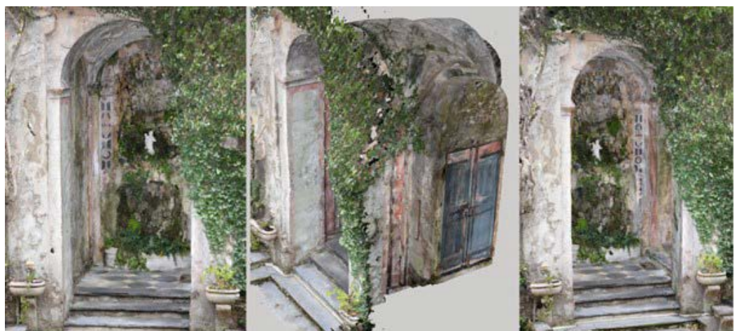
Fig. 10. Photogrammetric survey of the grotto - 3d model with texture. Elaboration by the authors.
