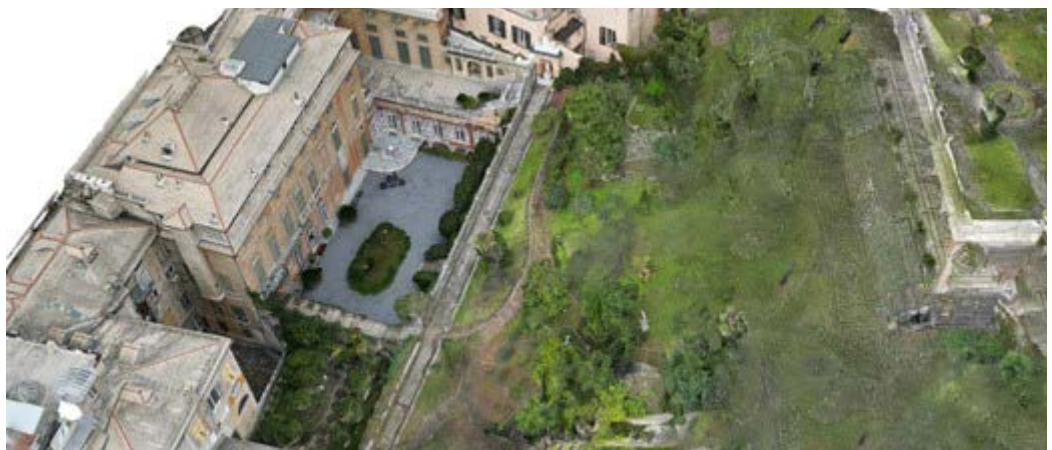
Fig. 12. Aerial photogrammetric survey of the palace and garden - 3d model with texture. Elaboration by the authors.
