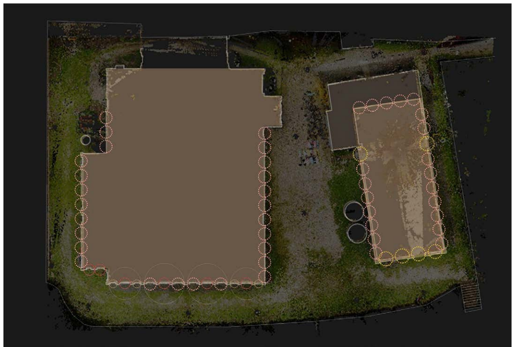
Fig. 6. Horizontal section of the point cloud with the different rhythms of the proportioning performed highlighted. Elaboration by the authors.
