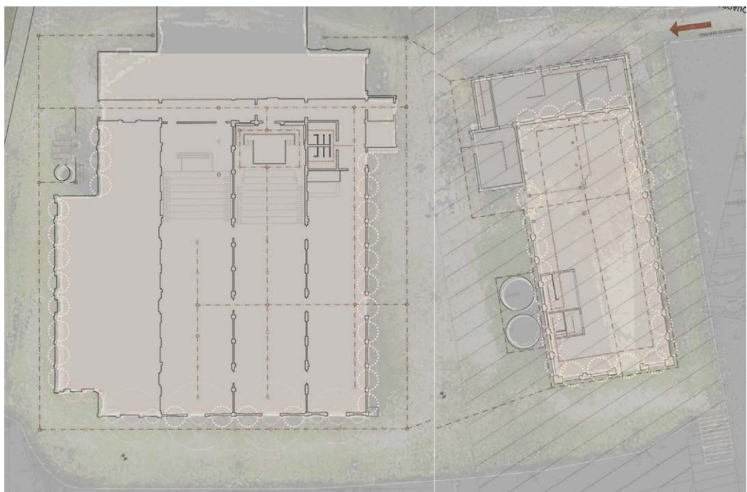
Fig. 8. Teatro India, overlapping of archive drawing in plan and point cloud. DSDRA archive drawing - Architectural survey scale 1:200. Course in Science of Representation III, students M. Caramella, F. Castelli, G. Decandia, a.y. 2005/2006, cad. drawing (ARDISCont 5.1). Elaboration by the authors.
