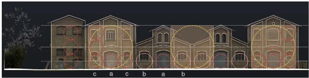
Fig. 7. Vertical section of the point cloud, detail of the south elevation of the main building, with the rhythms of the proportioning highlighted. In red is shown module A, in pink module B, in sepia module C, in orange three times module A. Elaboration by the authors.
