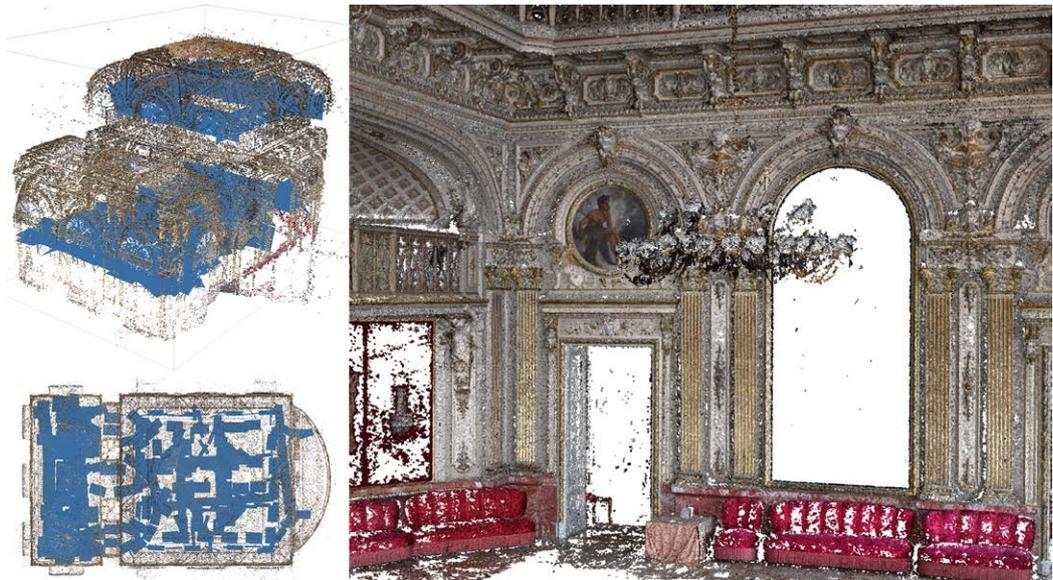
Fig. 4. Photogrammetric survey. Acquisition points of the photographic shots and perspective view of the point cloud. Elaboration by the authors.
