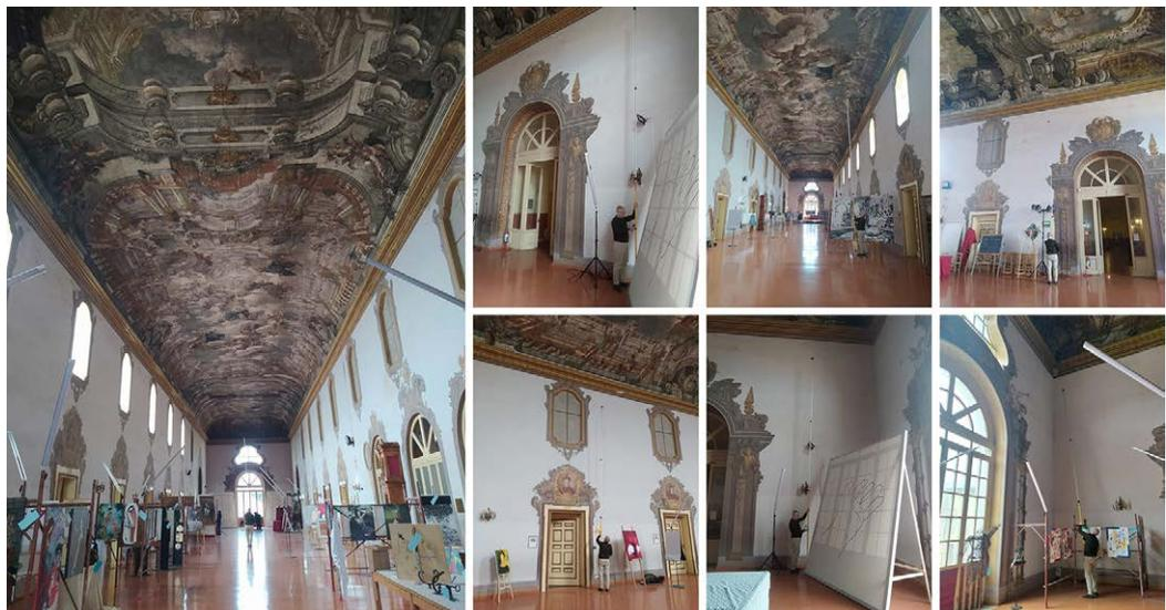
Fig. 5. Photographic documentation of the photogrammetric campaign phase. Dynamic shooting by means of Actioncam placed on a telescopic base.
