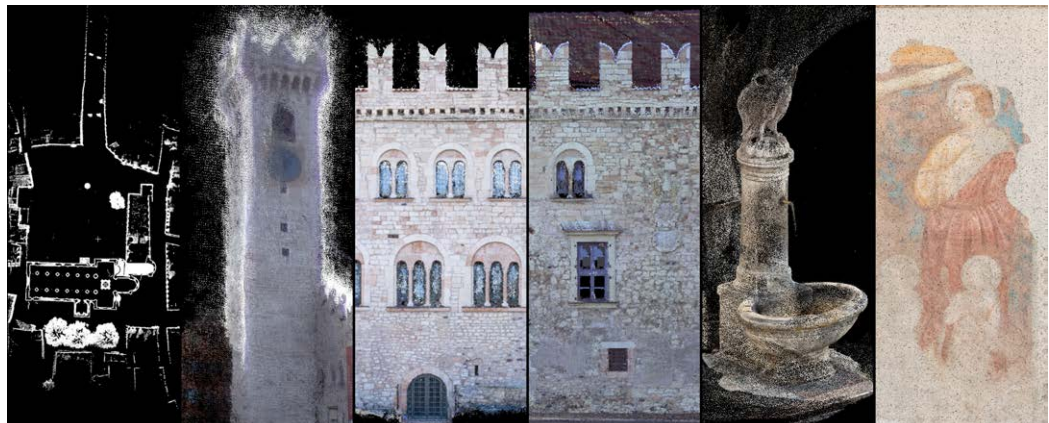
An evocative image showing the amount of data acquired using different 3D digital survey technologies. From left to right: mobile laser scanner, spherical camera, camera on a telescopic rod, terrestrial laser scanner; tablet with a LIDAR sensor; and drone. Elaboration by the authors.
