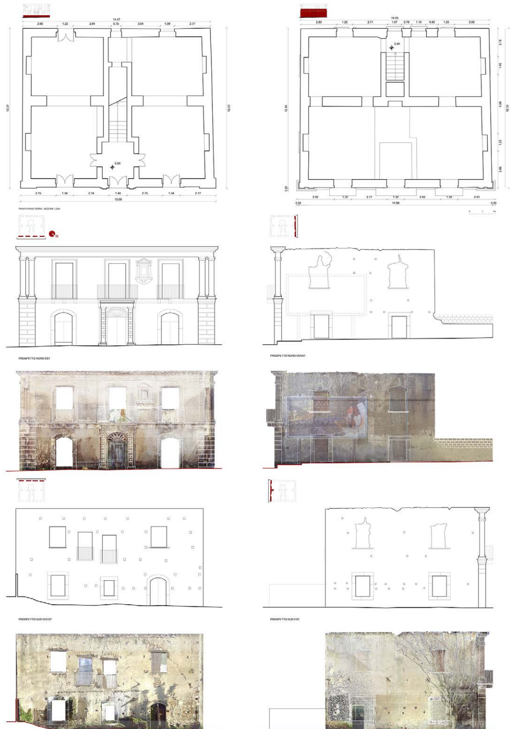
Fig. 7. Portanova Palace, Reggio Calabria. Drawing of elevations from laser scanning. Drawings made under the guidance of the author by Stefania Caporale, Francesca Maria Derenzo, Francesca Muscherà and Natali Sardone.
