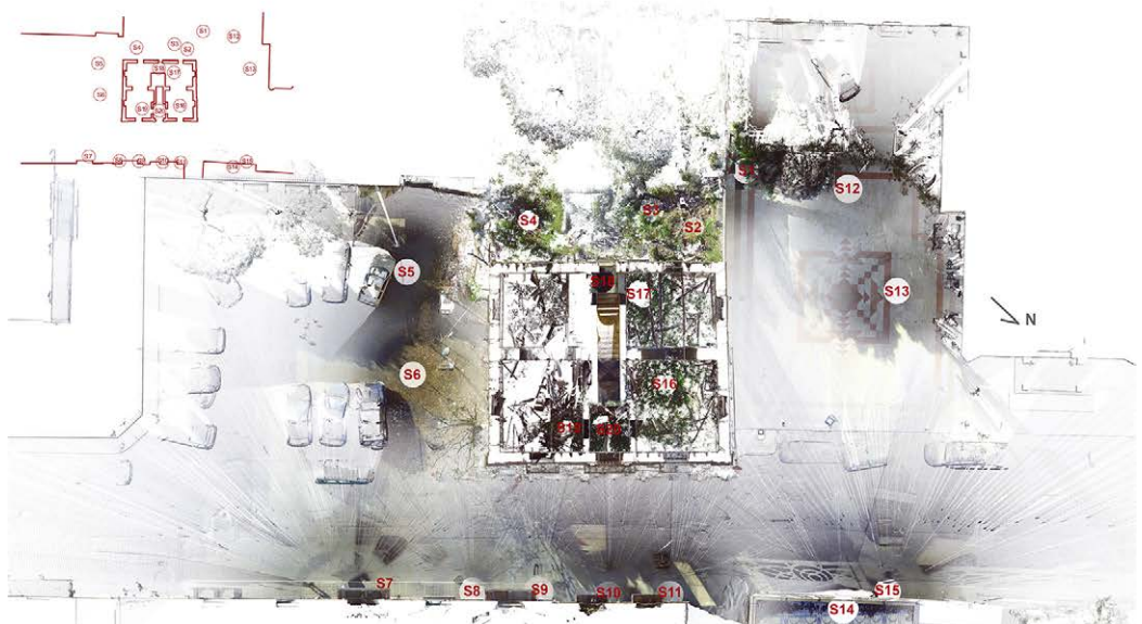
Fig. 6. Portanova Palace, Reggio Calabria. Workflow of the range based survey process. Drawings made under the guidance of the author by Stefania Caporale, Francesca Maria Derenzo, Francesca Muscherà and Natali Sardone.
