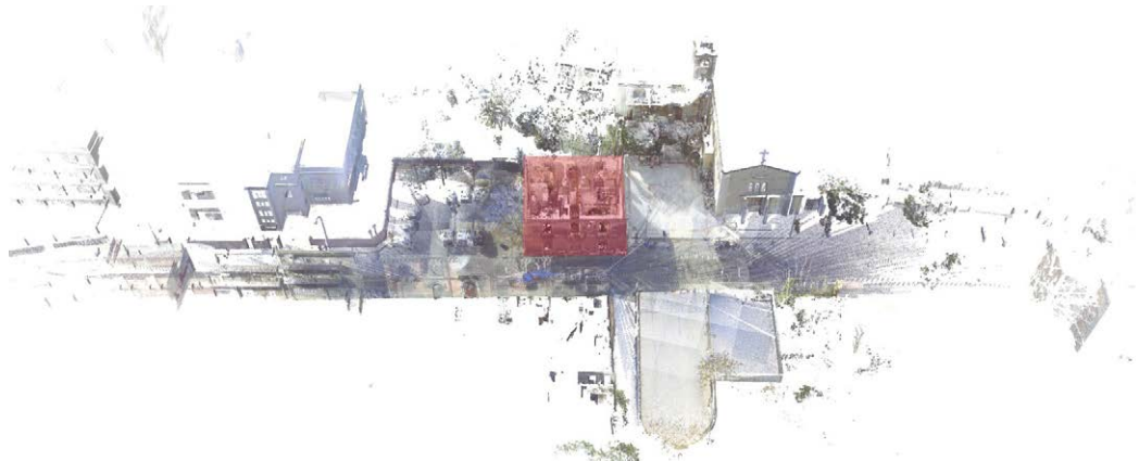
Portanova Palace, Reggio Calabria. Laser scan, point cloud of urban context.
