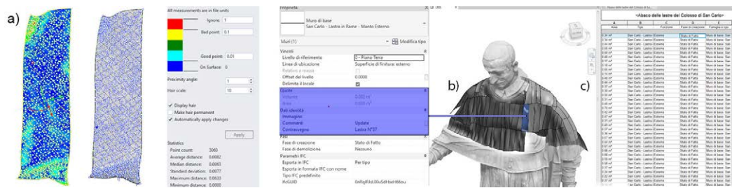
Fig. 7a. Curvature analysis and standard deviation. Fig. 7b. BIM objects and their properties. Fig. 7c. Copper plate schedule related to BIM parameters. Elaboration by the authors.
