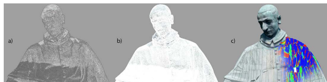
Fig. 6. Modeling process: a) from point clouds to b) mesh model and c) NURBS model and analysis of curvature (Gaussian). Elaboration by the authors.
