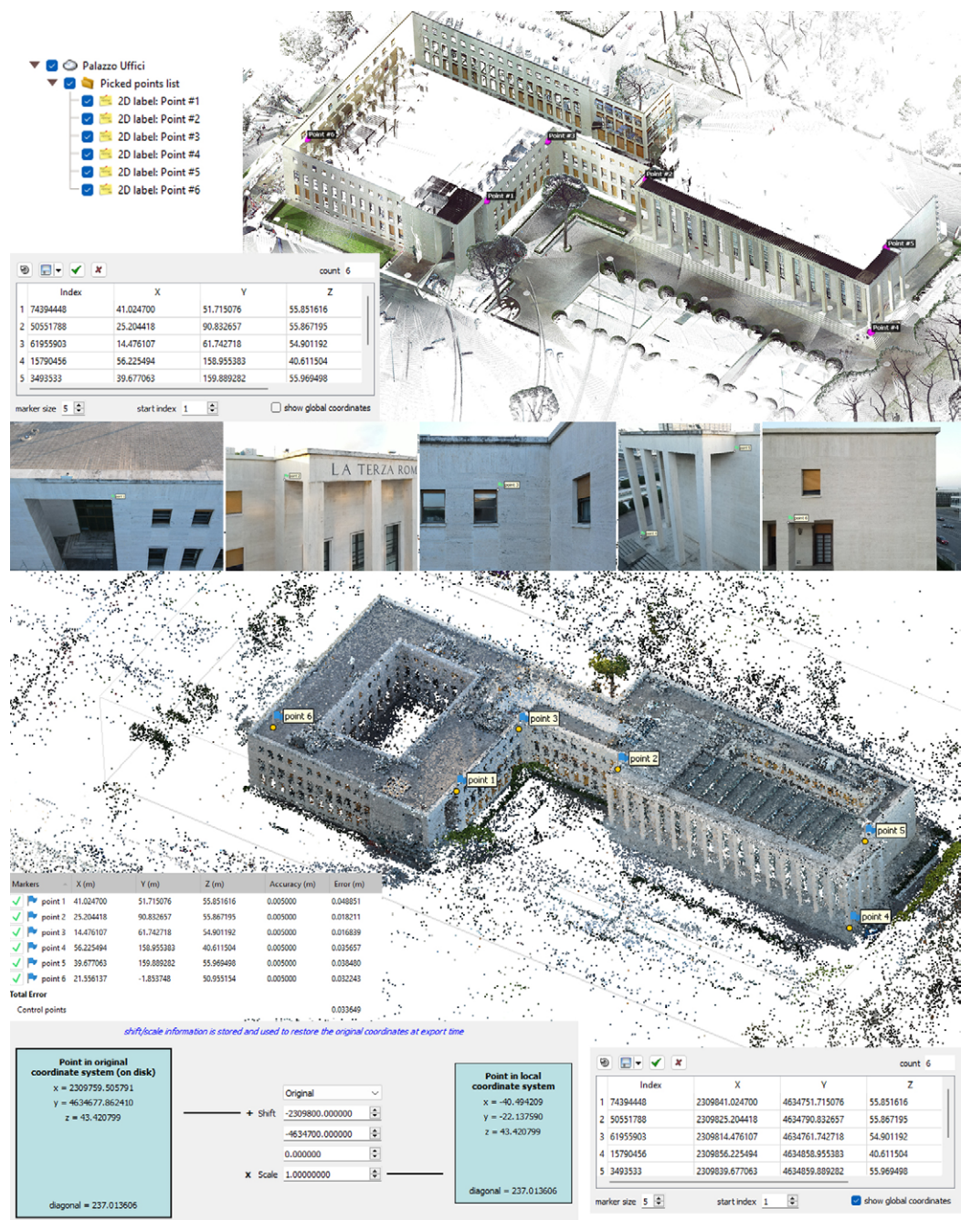
Fig. 3. Georeferencing of the IBM cloud (bottom) starting from some points with known coordinates - local and absolute - queried on the TLS cloud. Elaboration by the authors.
