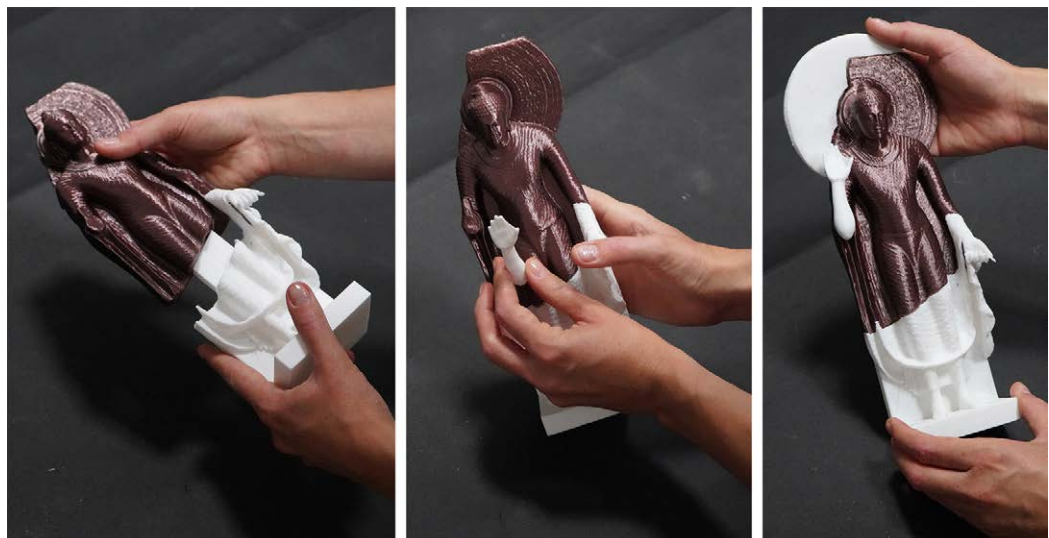
Fig. 3. 3D printed tactile replica Buddha: assembly of parts. Elaboration by the author.
