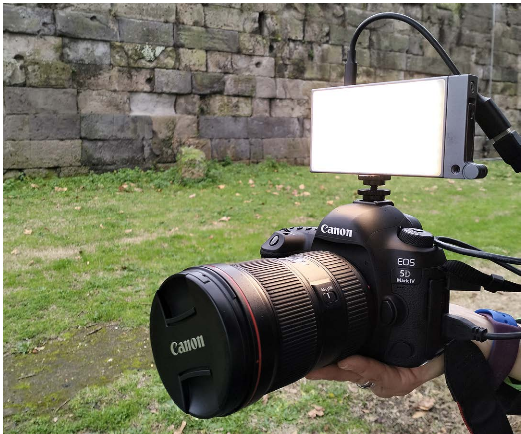
Fig. 2. Camera and illuminator used during the photogrammetric survey campaigns. Section of the ancient city walls chosen to demonstrate the methodology. Image by the authors
