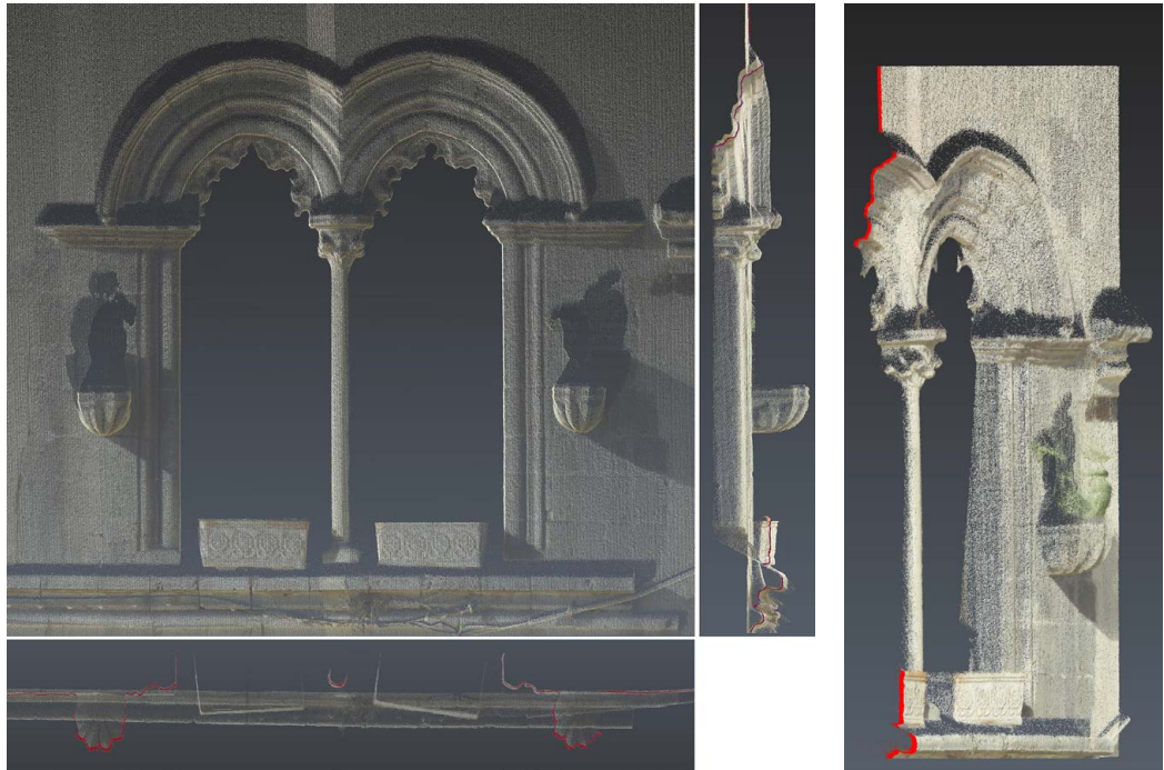
Fig. 10. Survey of the mullioned window in the historic center of Savoca (ME). Axonometric section. 3D model from the point cloud. Elaboration by the authors.
