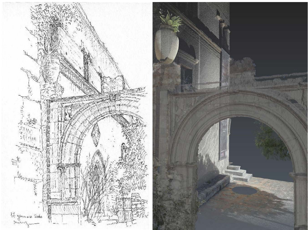
Fig. 12. Entrance arch of Palazzo Ciampoli in Taormina (ME). On the left: on sight survey. Drawing by Mario Manganaro; on the right: perspective view from the point cloud with mesh. Elaboration by the authors.
