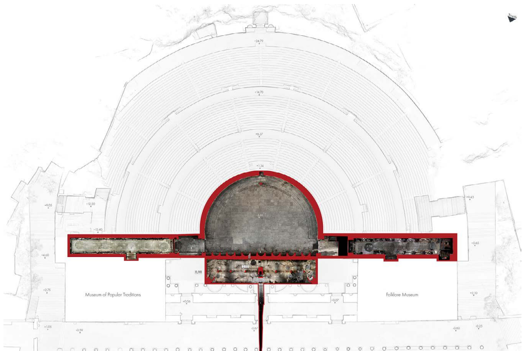
Fig. 3. Architectural survey of the theatre, plan and orthophoto showing the orchestra and the water piping under the building. Elaboration by Giuseppe Amoruso and Andrea Manti.
