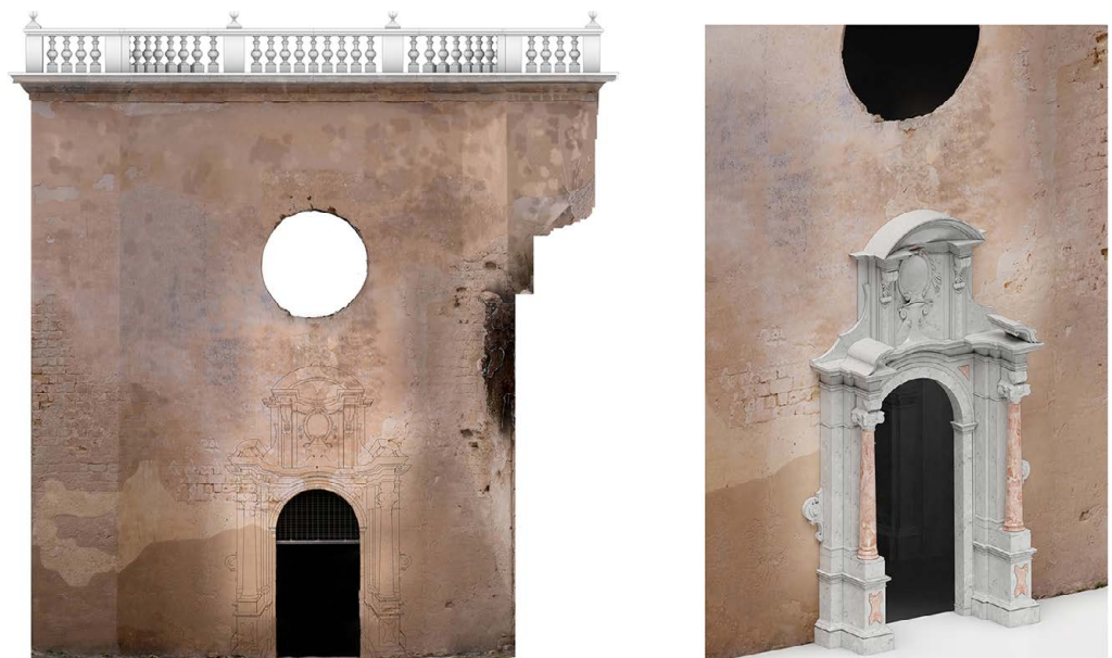
Fig. 12. Left: Hypothetical reconfiguration of the portal drawing. Right: Rendered axonometric view of the portal. Elaboration by M. Cannella.
