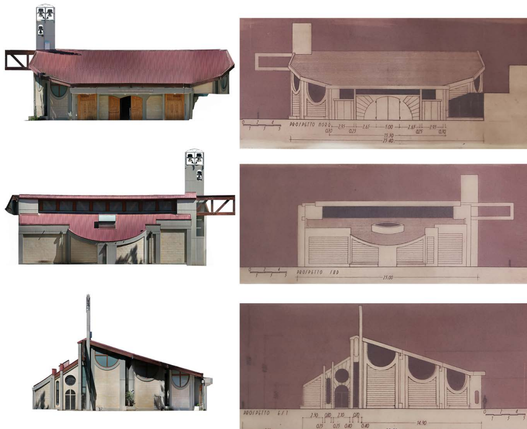
Fig. 2. Information layers of the Kühtz Archive. San Giovanni Battista Church: from the orthophotoplans of the north, the south and the east façades to the author's design drawings. Elaboration by F. Strippoli.
