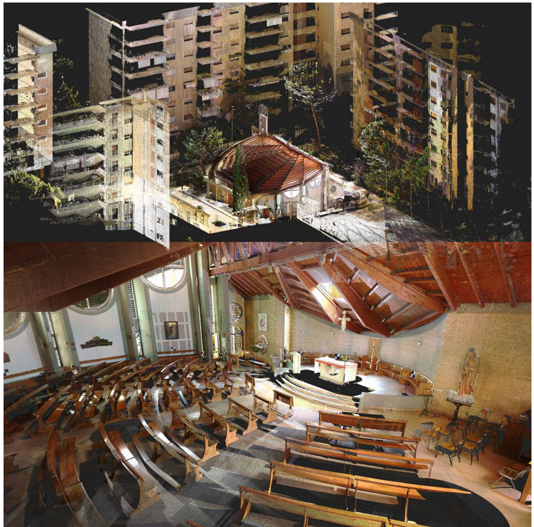
Fig. 4. Implementation of new data in the Kühtz Archive_San Giovanni Battista Church: three-dimensional model of the church from laser scanner point cloud. Elaboration by F. Strippoli.
