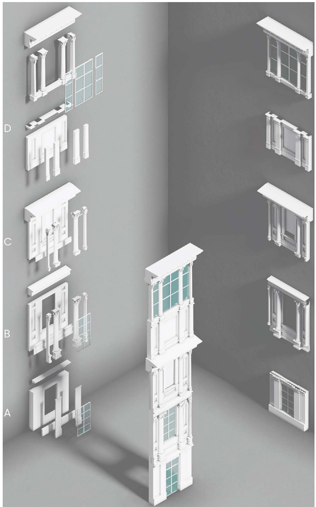
Fig. 7. "Dynamic model" of a part of the façade on five levels with an exploded view of the sub-components. Elaboration by L. Torresi.
