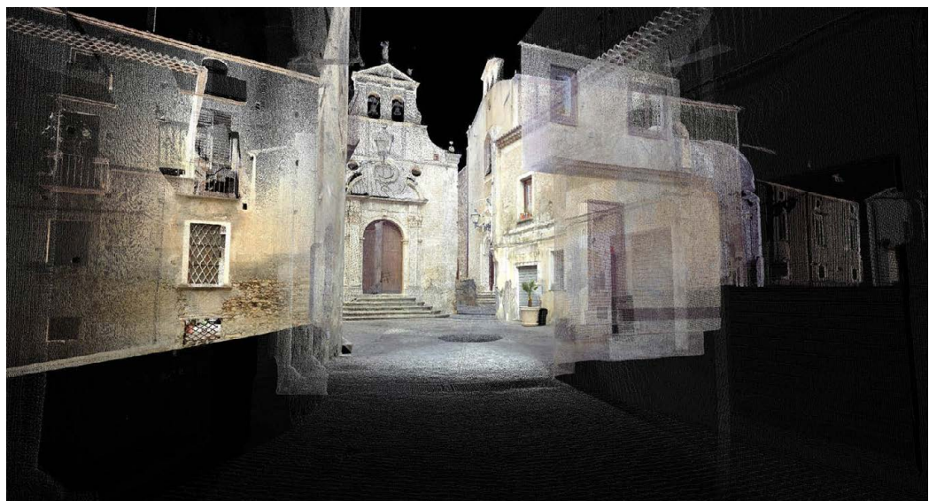
Fig. 6. The Church of the Addolorata, numerical model derived from laser scan processing. Elaboration of the authors.
