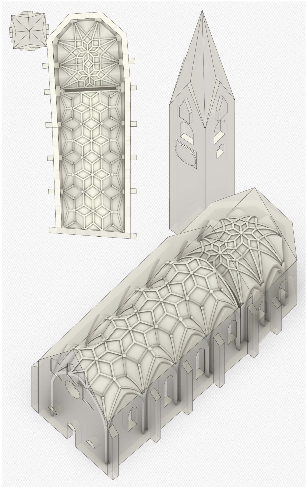
Fig. 8. Reconstructive hypothesis of the vaulted system based on the evidence from the survey data and the observations of related system. Floor plan and axonometric view. Elaborations by the authors.
