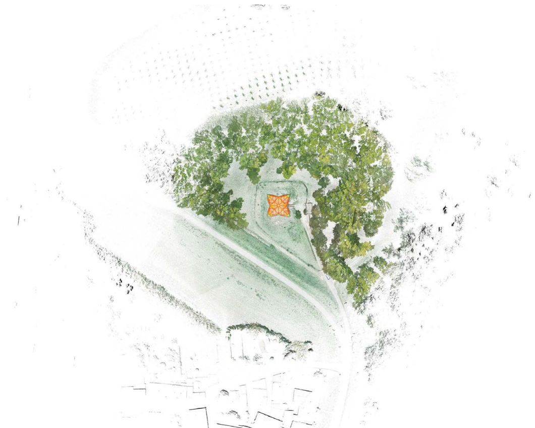
Fig. 4. Planimetric view of the point cloud obtained by aerial photogrammetry for the documentation of the landscape context of the Rocca in Stellata. Elaboration by the authors.
