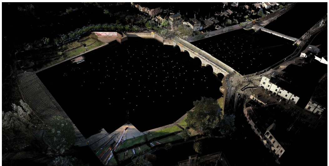
Fig. 6. The three-dimensional dataset of the Marecchia river basin integrates Laser scanner C10 and BLK data and photogrammetry. Elaboration by Guido Galvani.
