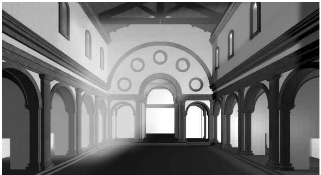
Fig. 9. Church of San Gallo. Reconstructive hypothesis of the interior; view towards the apse, trussed roof, clerestory with single-lancet windows. Elaboration by Ylenia Ricci.
