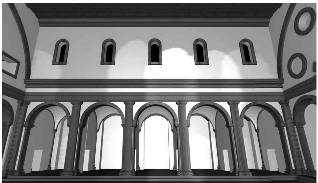
Fig. 10. Church of San Gallo. Reconstructive hypothesis of the interior; view of the chapels, coffered roofing, clerestory with single-lancet windows. Elaboration by Ylenia Ricci.
