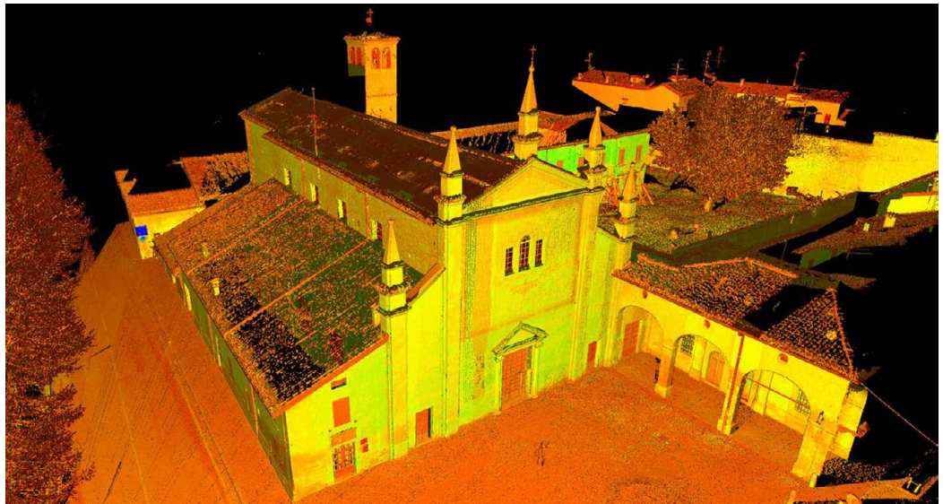
Fig. 5. Point cloud of the church obtained from the laser scanner survey. Graphic elaboration by the authors.
