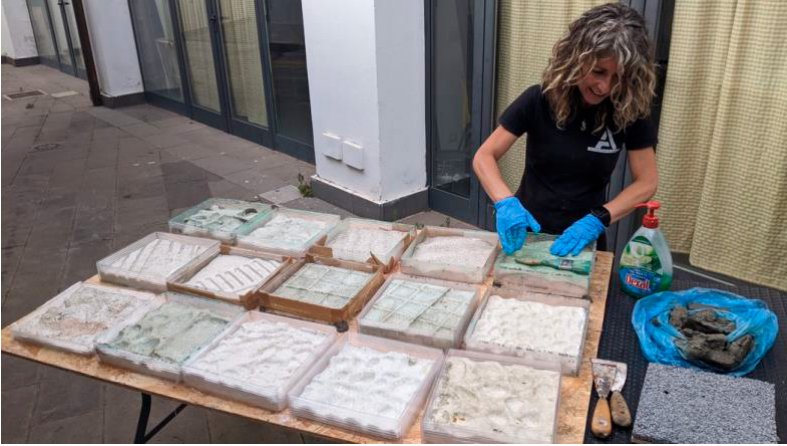
Fig. 5. Moulds obtained either directly from the original shapes and through a digital reproduction process. The final rubber tiles are obtained by pouring in the appropriate mould a rubber and resin compound. (lab. animazonedesign).
