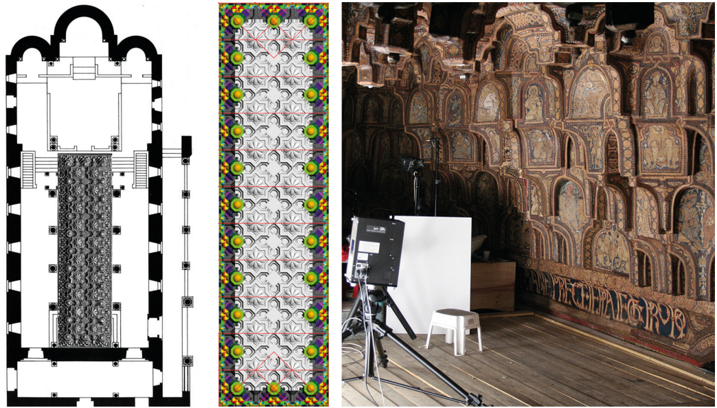
Fig. 2. Plan of the Palatine Chapel and orthogonal view of the ceiling's model; detailed view of the ceiling's model; surveying sessions from the restoration platform (photo and drawings by the authors).
