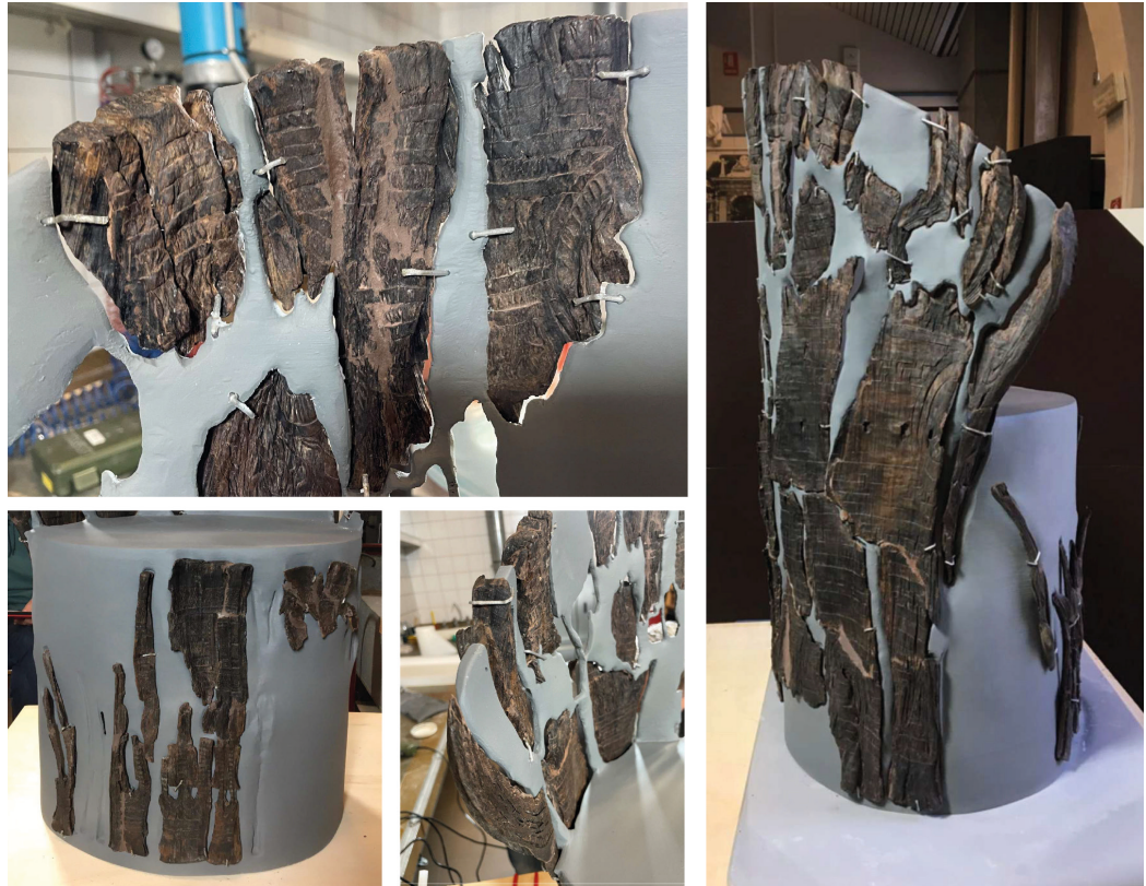
Fig. 6 Solid prototyping, fixing of the findings and reconstruction through anastylosis of the throne model (image by the authors).
