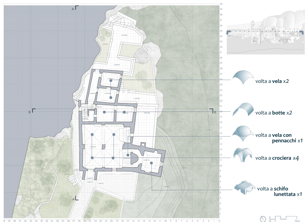
Fig. 9. Mapping of the vaulted roof systems of the Hermitage of Cetrella (image by the authors with C. Crati).
