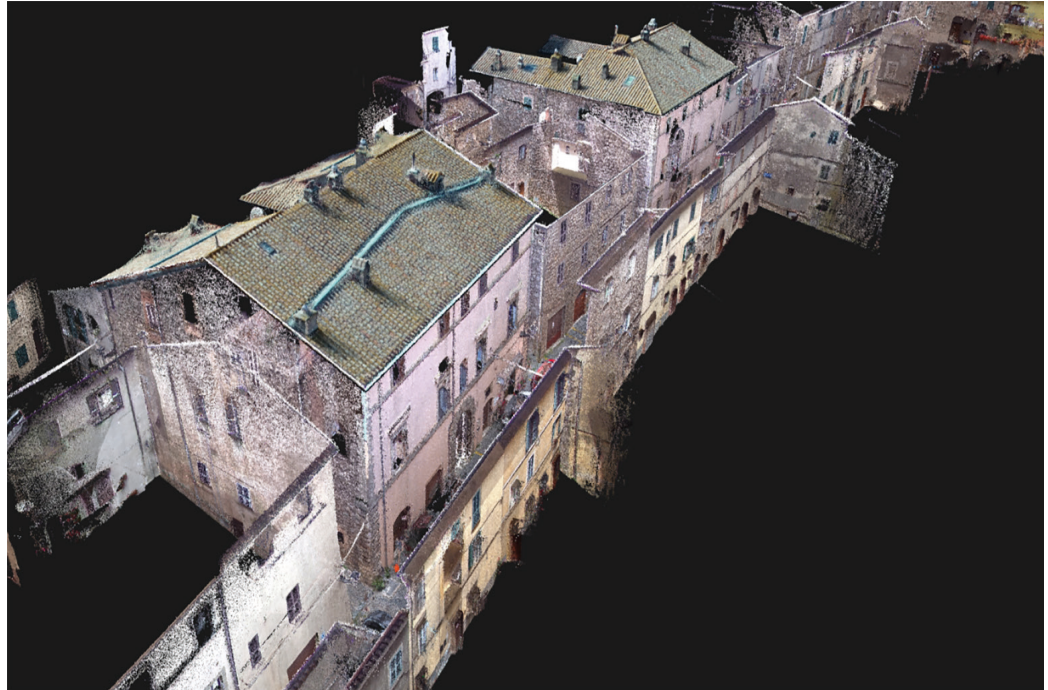
Fig. 6. Point cloud of the fronts and roof of Palazzo Panetti, together with a portion of Via Annibal Caro, created through the integration of data acquired with aerial photogrammetry, LiDAR and laser scanning (elaboration by the authors).
