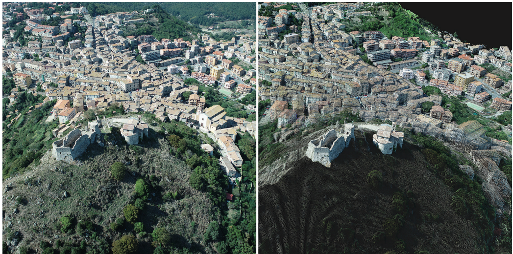
Fig. 10. On the left, view of Tolfa from the Frangipane fortress. Photo taken by Giuseppe Fioravanti with the camera mounted on the drone. On the right, view of the 3D point cloud model.
