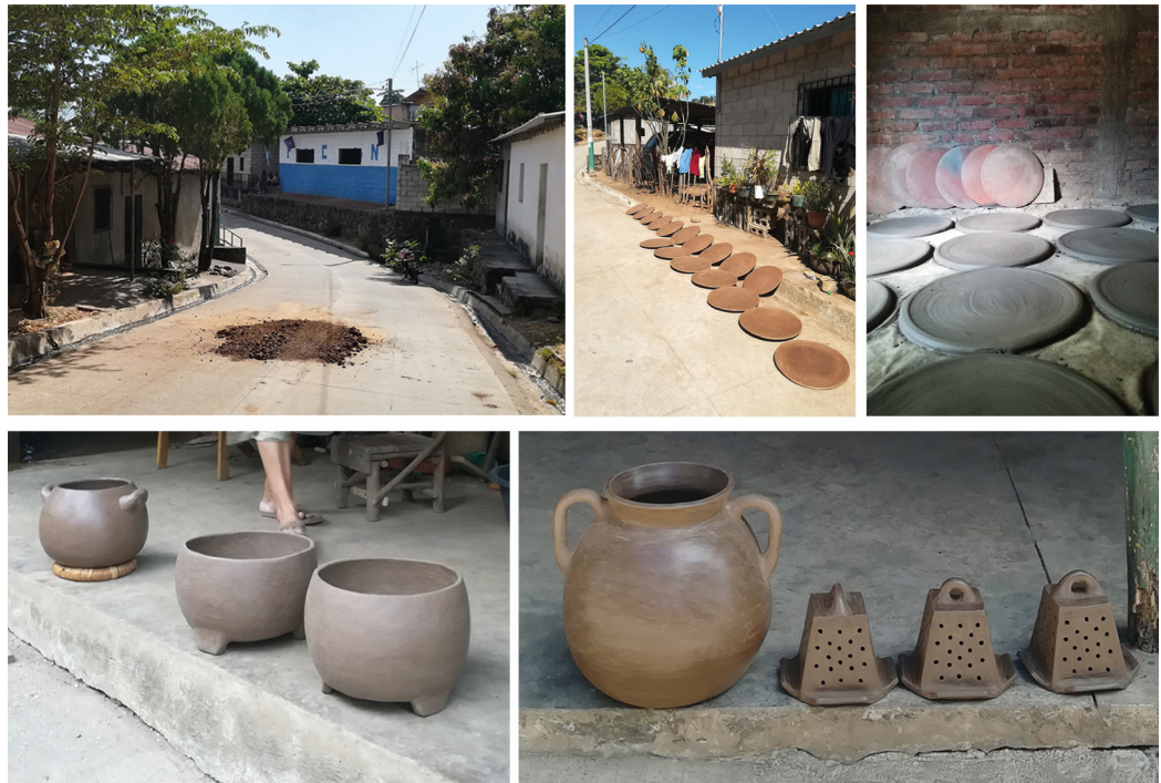
Fig. 6. Production phases of barro rojo artefacts. Pounding of the barro, processing, drying and baking (photo by the authors).
