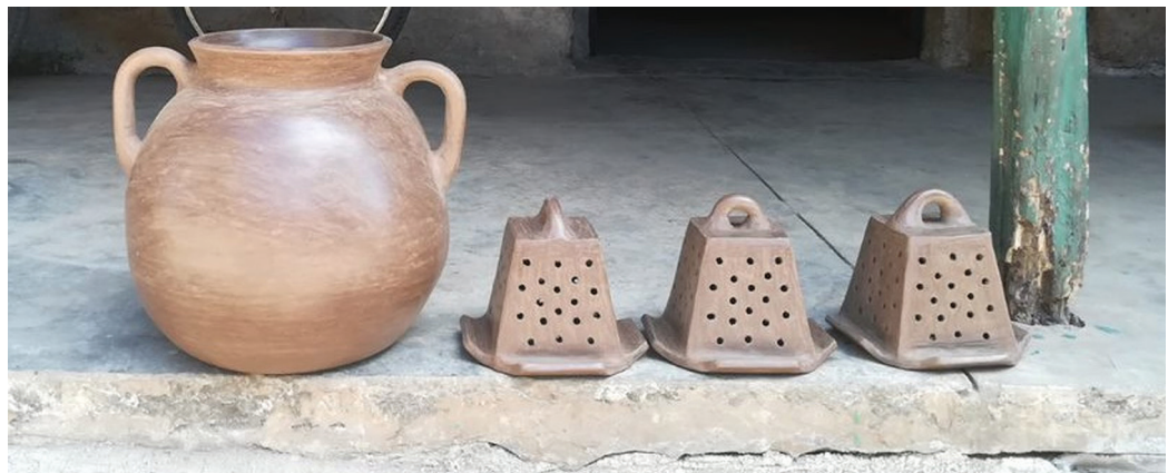
Handicraft products from the barro rojo chain. Casserole or pot and three toasters arranged for the natural drying of the clay (mud or barro in Spanish). Step prior to baking in a wood-fired oven (photo by the authors).
