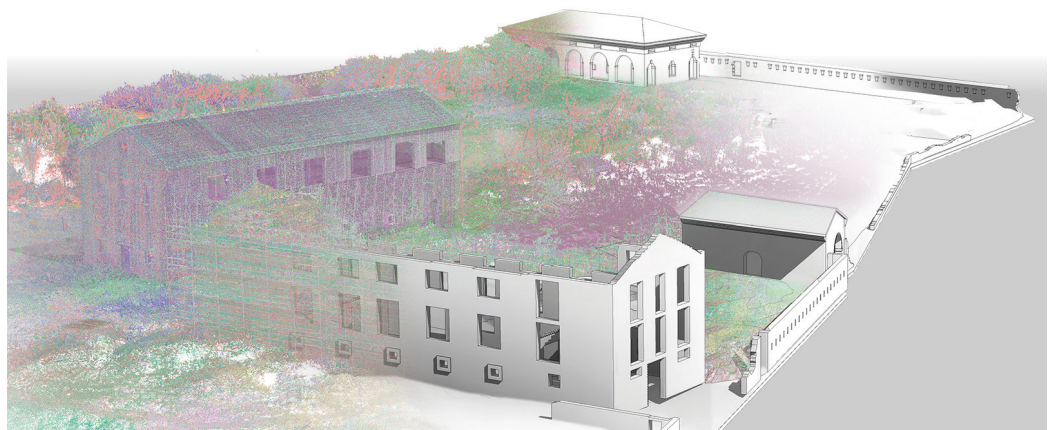
Conceptual outline of the scan-to-BIM process of parametric model restitution.
