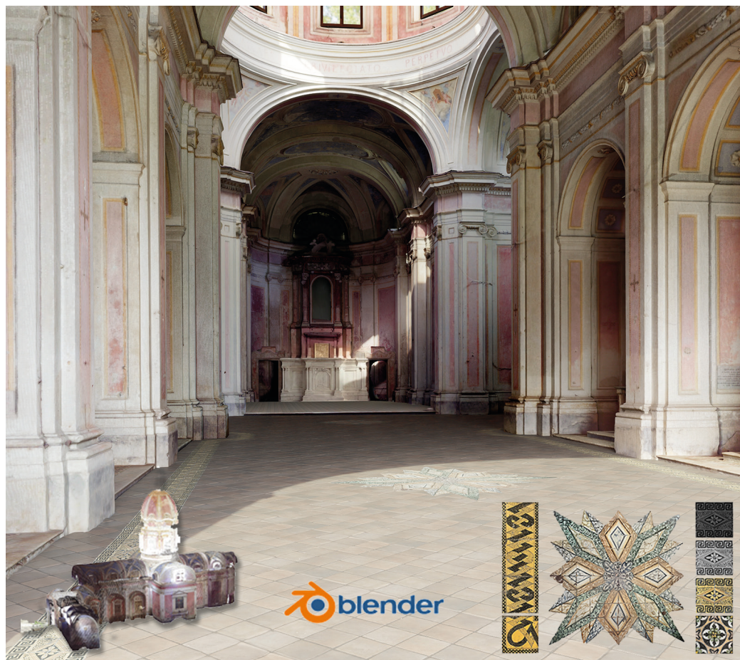
Fig. 9. From the point cloud model (edited by Rosina Iaderosa) to the explorable digital model developed with a sculpting phase for partially occluded areas such as details of the majolica flooring and some chapels (edited by C. Di Rienzo).
