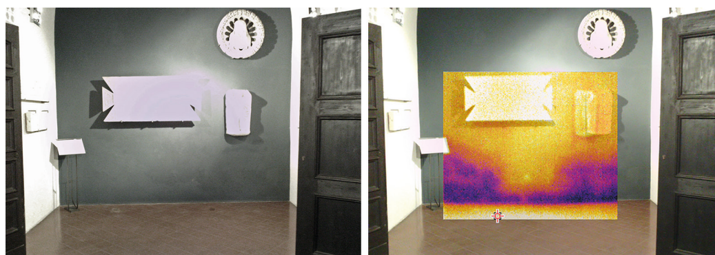
Fig. 11. Thermographic survey with overlay of the two channels, photographic RGB and thermographic, captured by the instrument. The presence of an opening beneath the plaster layer can be observed.
