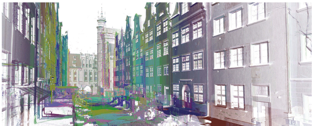
Alignment and merging of multiple scans to create a unified 3D representation.
