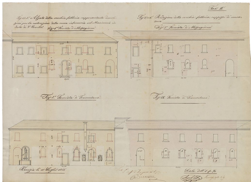
Fig. 3. Elevations of the 18th-century building transformed into an infirmary, indicating the works carried out, 1866, (ASVe, Civil Engineering Office, Records, b. 737, drawing 9).
