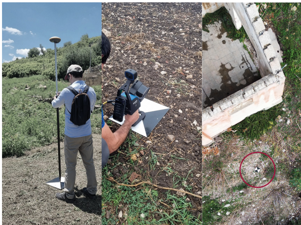
Fig. 5. Acquisition of markers in the GNSS, SLAM and photogrammetric survey.
