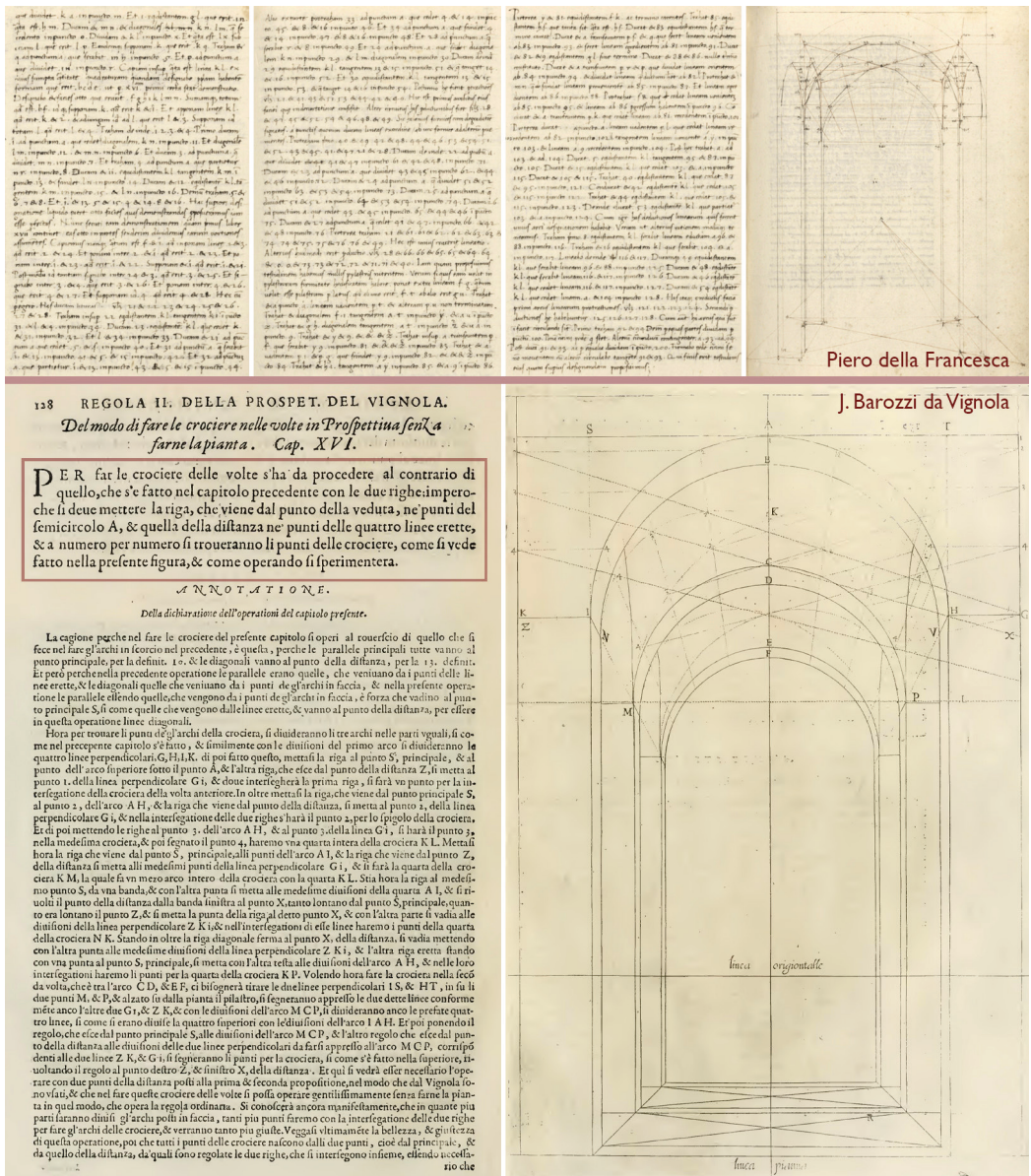
Fig. 2. Describing the drawing: the relationship between text and image in the representation of a groin vault in Piero della Francesca's De prospectiva pingendi (top) and in Vignola's De due regole (bottom). Vignola (text in the inset) entrusts the figure almost entirely with the task of evoking the construction process.
