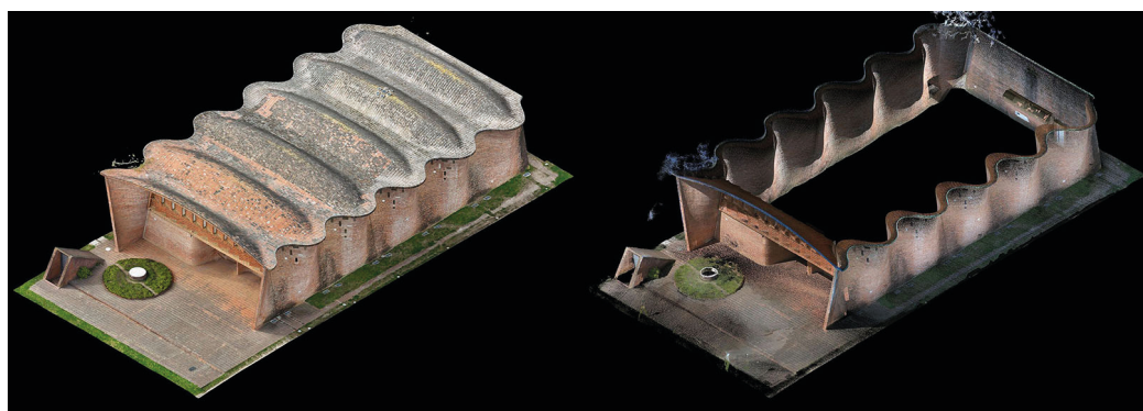
Fig. 8. RGB visualization of photogrammetric point cloud (left) and SLAM XGRIDS Lixel KI point cloud (right) (elaborations by the authors).
