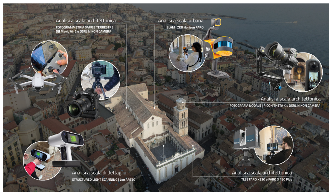
Fig. 2. The digital survey technologies used to generate the multi-scale information database: the SLAM ZEB Horizon FARO mobile laser scanner, the DJI Mavic Air 2, the Nikon D800E DSLR cameras, the Ricoh Theta X camera, the FARO X330 and S 150 Plus terrestrial laser scanners, and the Leo ARTEC structured light scanner.
