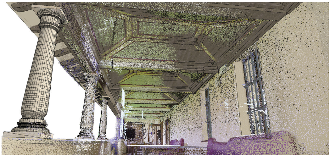
Fig. 9. HBIM model Charterhouse of Pesio. Screenshot model overlaid with point cloud (elaboration by the author).
