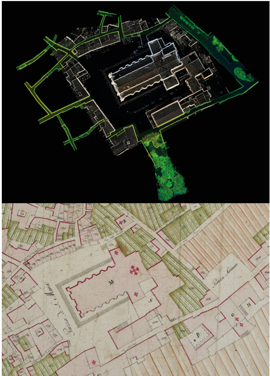
Fig.10 Result of the integrated survey combining UAS systems (Cathedral exterior), a Faro Focus S70 scanner (Cathedral interior) and a NavVis VLX 3 device (context). Compared with the first parcel cadastre of the Papal State, initiated by Pius VII in 1816 and enacted by Gregory XVI in 1835. Detail of the Gregorian Cadastre sheet for Orvieto Cathedral. Source: image by the authors and www.imagoarchiviodistatoroma.cultura.gov.it
