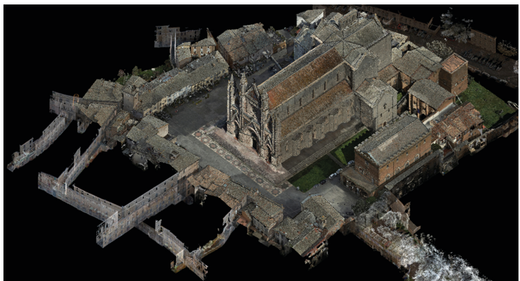
Fig.9 Outcome of the integrated survey combining UAS systems (Cathedral exterior), a Faro Focus S70 (Cathedral interior) and a NavVis VLX 3 (urban context) (image by the authors).
