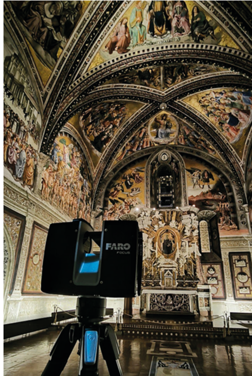
Fig.5 Left: scan of the Chapel of San Brizio with a Faro Focus S70. Right: scan of the cathedral square with a NavVis VLX 3 (images owned by the authors).
