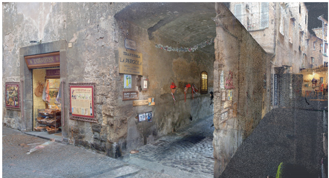
Fig.8 Overall dense point cloud of Orvieto's historic centre and a close-up of a narrow lane, generated by the NavVis VLX 3 survey (image by the authors).
