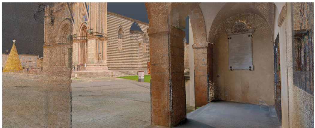
Point cloud of the Orvieto Cathedral context generated with the NavVis VLX 3 mobile laser scanner (image by the authors).
