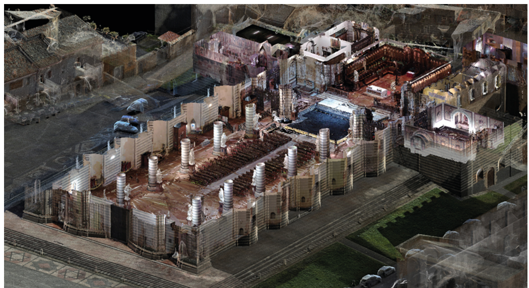
Fig.7 Dense point cloud of the Cathedral interior in section, scanned with a Faro Focus S70 and embedded within the wider Orvieto context captured by drone and NavVis VLX 3 (image by the authors).
