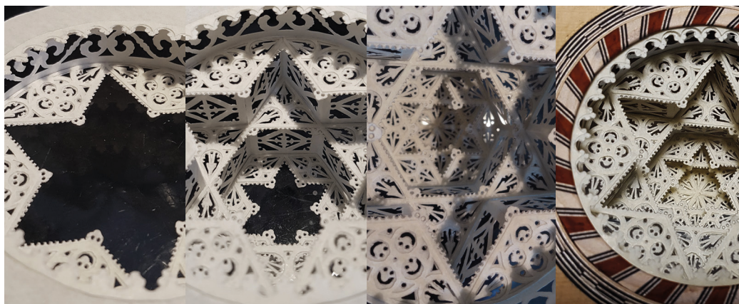
Stages of making the parchment rosette and frame of the soundhole on the soundboard (photo by the author).
