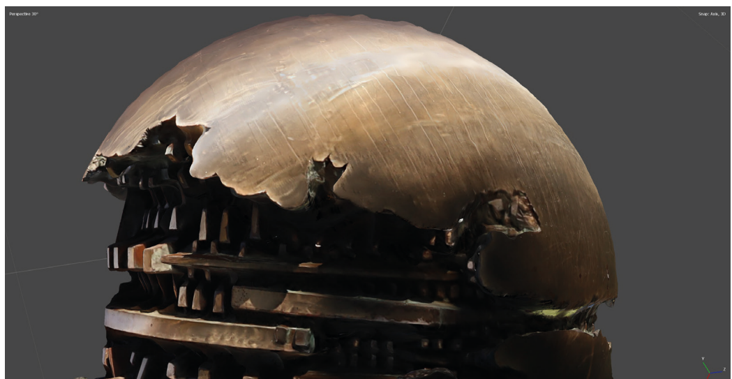
Fig. 9. Sfera grande by A. Pomodoro, Pesaro. Portion of the corrected model, complete with mesh and texture, showing the efficiency of photogrammetry systems in acquiring and representing the surface condition (image by the authors).
