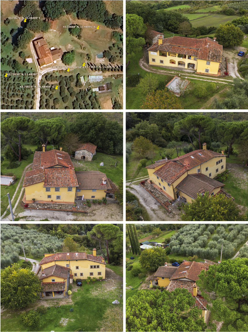
Fig. 2 Examples of photos taken from drone during the survey campaign, with detection of the coordinates of the photo shooting points (elaboration by the authors).
