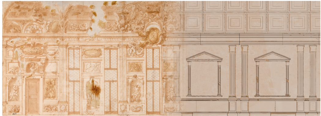
Fig. 10. Comparison between the reference image (Domenico Piola, Design for ceiling and wall frescoes , c. 1684) for shading style and the result achieved so far (authors' drawing). The latter consists of multiple procedural textures that vary depending on the light source's position.
