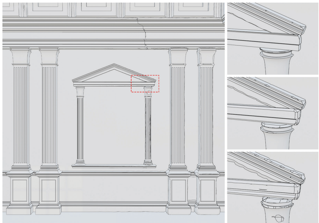
Fig. 9. Transition to a ruined model through edging. The parametrization of shapes via VPL allows for a gradual adjustment of this effect (authors' drawing).
