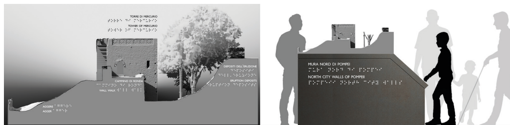
Fig. 10. Section of the model from Fig. 9 showing terrain elevation changes, with simplified explanations of architectural elements, including Braille labels for blind and visually impaired users and the installation of the model on a display support for use in a museum space (elaboration by S. Bertacchi).
