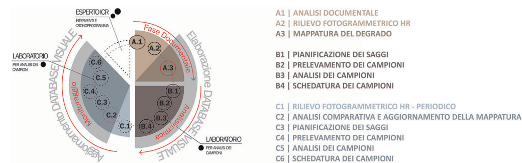
Fig. 8. Diagram of the proposed process for analysis, diagnostic planning, and monitoring (graphic elaboration by the authors).
