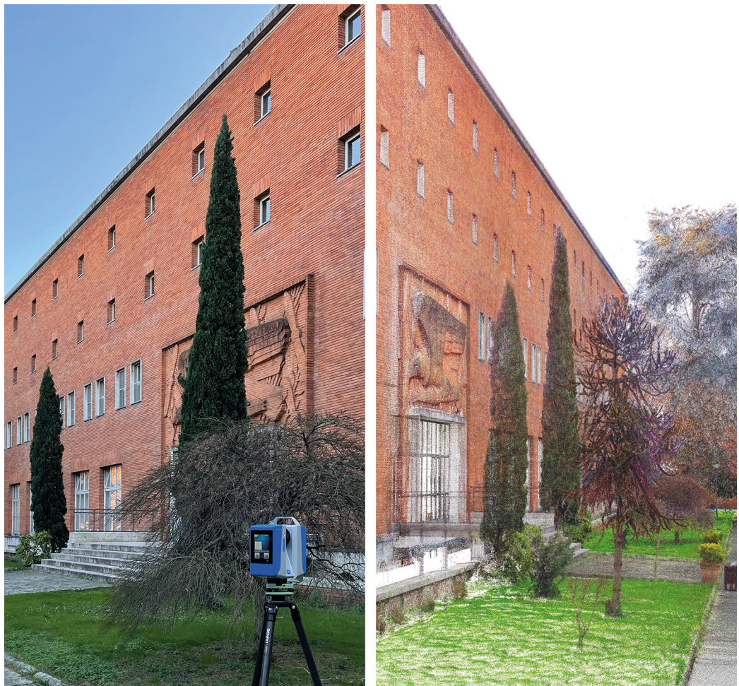
Fig. 3. Data acquisition phases using TLS and view of the colored point cloud of the Palazzina Ufficiali (photo and graphic elaboration by the author).
