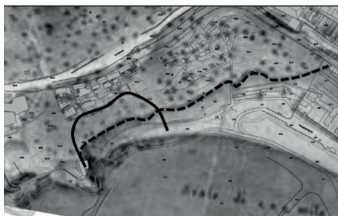
Figure 7. The upper edge of the Calanco in 1826 is in dashed gray, the current edge in black. The lower edge of the Calanco in 1826 is in dashed dark gray, the current edge in black
