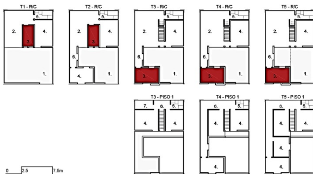
Figure 3 - Plan with all typologies, version A, of the year 1977. 1. Patio, 2. living room, 3. kitchen, 4. bedroom, 5. sanitary installation, 6. circulation, 7. storeroom
