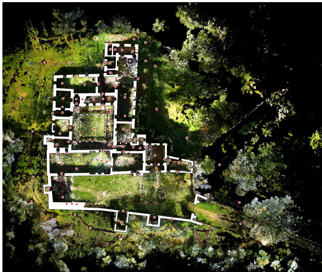
Figure 3 - General plan from point-cloud with indication of the stations of the laser-scanner survey
