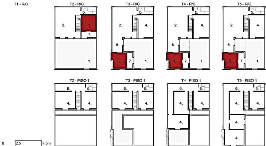
Figure 7 - Plan with all typologies version Ac, of the year 1980. 1. Patio, 2. living room, 3. kitchen, 4. bedroom, 5. sanitary installation, 6. circulation, 7. laundry
